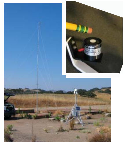
RSR2™ system with 10 meter wind sensor pole mount (primary irradiance sensor in cutout)
